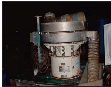
STOCK CODE: N10284-16 600MM DIA S/S SWECO SINGLE DECK SIEVE TYPE LS24-S-44. DRIVEN BY 0.25KW MOTOR
