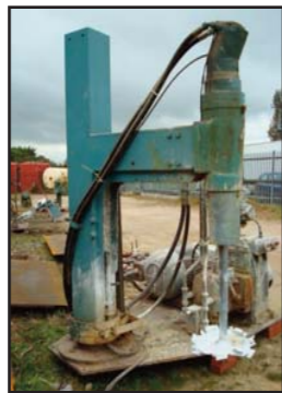
STOCK CODE: N10050-03 37KW TORRANCE HYDRAULIC RAISE/LOWER SAWTOOTH MIXER
