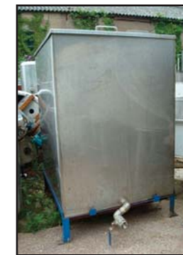
STOCK CODE: N10314-07 1400L S/S RECT. TANK 1000 X 1200 X 1300MM TALL
