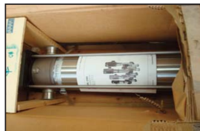
STOCK CODE: N10353-33 160 LPM GRUNDFOS PUMP TYPE CRN10 S/S
