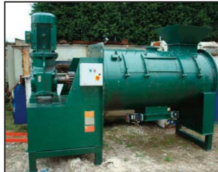
STOCK CODE: N10137-10 1000L S/S WINKWORTH RT1000 S/S 30KW T-ARM BATCH MIXER
