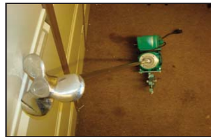
STOCK CODE: S9468-03 1.1 KW CLAMP ON STIRRER 1440 RPM
