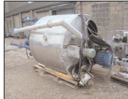
STOCK CODE: N10317-02 2100L S/S ENC COMBINATION MIXING TANK 1560MM DIA X 1200MM DEEP. DISH BOTTOM
