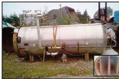
STOCK CODE: N8181-06 4600 L M/S HORIZONTAL AUTOCLAVE 50 PSI
