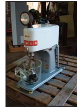
STOCK CODE: N9622-50 0.25KW WEMCO SHEARHEAD STIRRER
