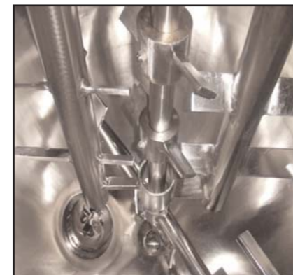
STOCK CODE: N10326-01 500L S/S GIUSTI SCRAPED SURFACE MIXER FULL VACUUM/1 BAR. TEST PRESSURE 1.5 BAR
