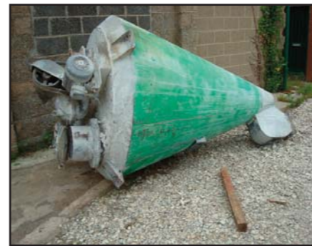
STOCK CODE: N10301-10 1250L S/S NAUTA MIXER WITH ORBITAL MIXER SCREW 1800MM DIA X 2200MM TALL
