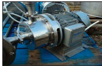
STOCK CODE: N10085-03 4KW S/S MORITZ TR100 INLINE SHEAR MIXER
