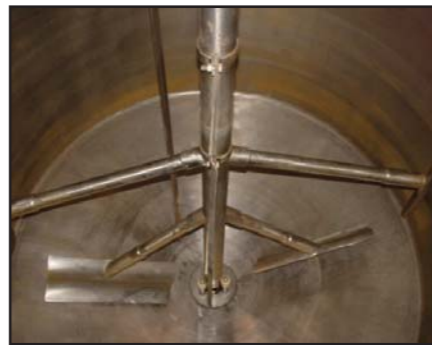
STOCK CODE: N10313-01 6250L S/S VERTICAL JACKETED MIXING TANK 2000MM DIA X 2000MM DEEP
