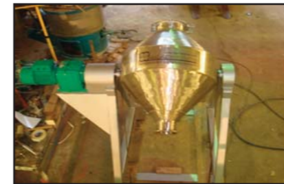
STOCK CODE: N7366-10 110L S/S DOUBLE CONE BLENDER 1.5KW
