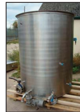
STOCK CODE: N10332-07 2750L OPEN TOP MIXING TANK S/S 1500MM X 1870MM DEEP
