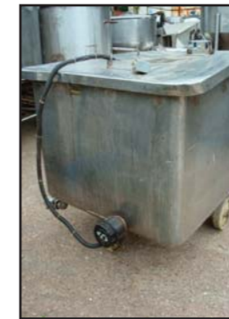
STOCK CODE: N10315-04 700L S/S ELEC. HEATED RECT. TANK 900MM X 1280MM X 700MM DEEP
