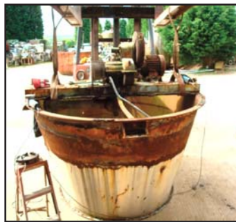
STOCK CODE: N9442-10 5000L MILD STEEL NAUTA MIXER 2200MM DIA X 3600MM TALL WITH PLANETARY AUGER MIXER CONVEYOR WITH BASE MOUNTED AIR OPERATED SLIDE VALVE PRODUCT DISCHARGE
