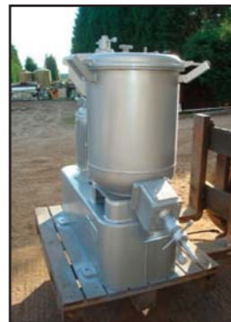
STOCK CODE: N9849-09 70L S/S STEELE COWLISHAW 11KW HIGH DISPERSION MIXER
