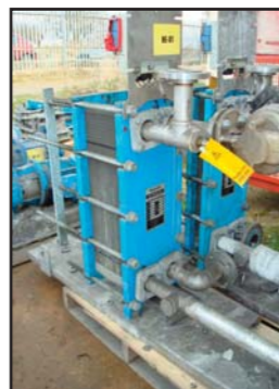
STOCK CODE: N9928-19 16 SQ.M. RYCROFT PLATE HEAT EXCHANGER
