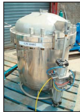
STOCK CODE: N9977-06 130L S/S VERTICAL AUTOCLAVE T.P. 8 BAR
