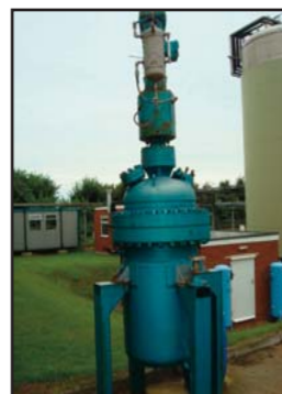
STOCK CODE: N5768-01 300 L S/S HIGH PRESSURE JACKETED REACTOR
