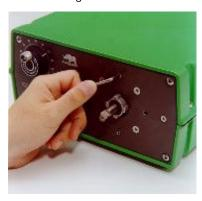
Fit the track in any one of three orientations, over the drive shaft and locating boss. Secure the track with the locating screw. Ensure the drive shaft is degreased before locating the rotor onto the shaft via the split collet. Tighten the rotor screw to a torque of 3Nm to prevent the collet slipping during operation.
