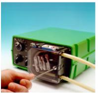
Fit the other end of the tubing into the second spring loaded clamp, ensuring that the tubing is not slack in the pumphead, since this can reduce tube life.
