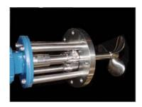
RIGAL BENNETT GROUP - SE range of side and bottom entry mixers. Our high quality low maintenance design is suitable for low to medium viscosity mixing in mixer tanks from 4,000L to 100,000L capacity. Our mono block mixer is designed for flange mounting with seals to suit individual application. All contact parts are 316 grade stainless steel.
