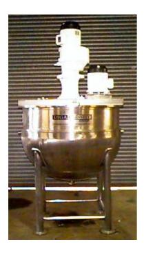
RIGAL BENNETT GROUP – KM range of scraped surface mixers are used for a large number of applications where mixtures need to be stopped from sticking to the heated or cooled side of the mixer. All contact parts are 316 grade stainless steel and scrapers are ptfe plastic.
