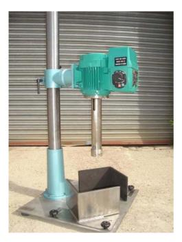
**RIGAL BENNETT** range of laboratory mixers are simply designed for bench use, and can be mounted on stainless steel stand with adjustable clamps. A range of agitators are available and all contact parts are 316 grade stainless steel.
