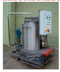
RIGAL BENNETT - We have a range of stainless steel tanks designed for liquids up to 1.3 specific gravity. Units have stiffened top ring to accommodate a clamp stirrer or bridge mounted.
