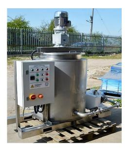
RIGAL BENNETT OJ range of stainless steel tanks is designed for liquids up to 1.3 specific gravity. Units have stiffened top ring to accommodate a clamp stirrer or bridge mounted.
