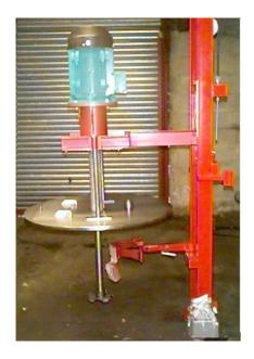
RIGAL BENNETT GROUP TH-range of saw tooth dispersion mixers are used for countless applications for wet milling, emulsifying and mixing of low to high viscosity fluids.
