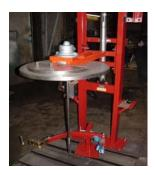
RIGAL BENNETT DM range of mixers is designed for low to medium viscosity mixing. Units can be clamp, screw, bridge or crane mounted. Agitators for fitting to 1220 mm maximum length shaft are marine or centripetal propeller, turbine or single paddle. All contact parts are 316 grade stainless steel.
