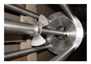
This special mixer is designed to give intensive mixing, simultaneous deep dispersing and emulsifying action, with a new double acting Duplex head which is specially designed with no bearings immersed in the process solution. This design enables mixing times to be dramatically reduced from conventional stirrers by up to 75%. The mixer design has the following features:-
