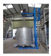
RIGAL BENNETT fixed raise/lower units are used with a number of mobile tanks to enable one mixer to mix several tanks
